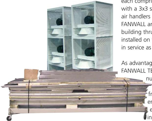
**Specifying knock-down construction for the air handler with FANWALL TECHNOLOGY makes it easy to fit the pieces inside an existing building and avoid expensive demolition. Disassemble the AHU on site or have it arrive already disassembled as shown above. FANWALL cells fit through standard width doorways.**
