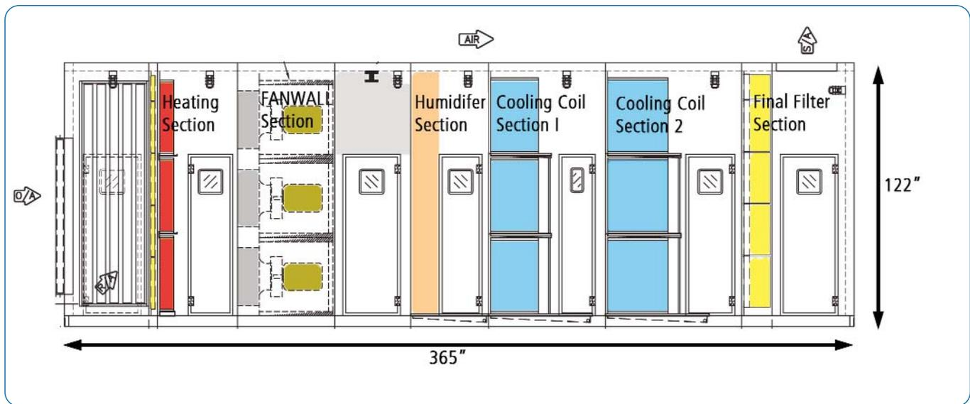
**Elevation view of Ventrol knock-down air handler with a 9-fan FANWALL array for hospital retrofit. Designed to deliver 38,000 CFM @ 12-inches total static pressure.**
